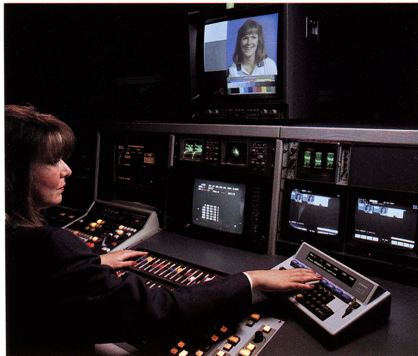
ESS-5T systems enhance color correction in film-to-tape transfer applications. (Photo courtesy The Post Group)
